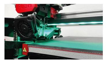
Adjust the distance between the nozzle and the heatbed with the knurled bolt to 0.8 mm by following steps:
