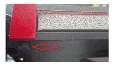
Loosen the screw from Z-axis slider (1) and use knurled bolt (2) to lower a slide a few millimeters (clockwise), in order to move the hotend from the heatbed (for safety).
