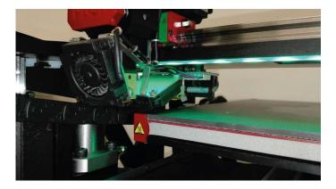
Move the heatbed slowly to the front to such position that the hotend is above the front left corner of the heatbed – be careful so the heatbed do not hit the hotend (hotend should be a few milimeters above the heatbed).
