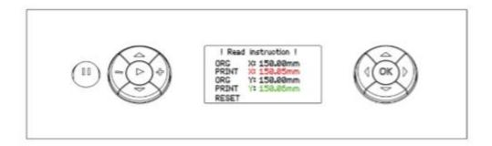
Due to this procedure, the next printout from the material, for which the calibration was made, will be completed with the compensation for thermal contraction of the material in X and Y axes
