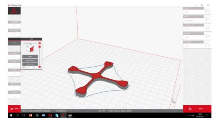
After printing, cooling and careful removal of calibration object (the cross), take measures of X and Y axes of the printed model. Several measuring tools can be used, provided that their accuracy cannot be worse than 0.05mm:
