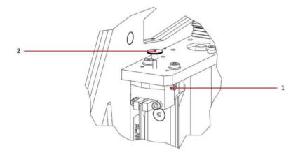
Fig. 30. Hotend height adjustment screws.
