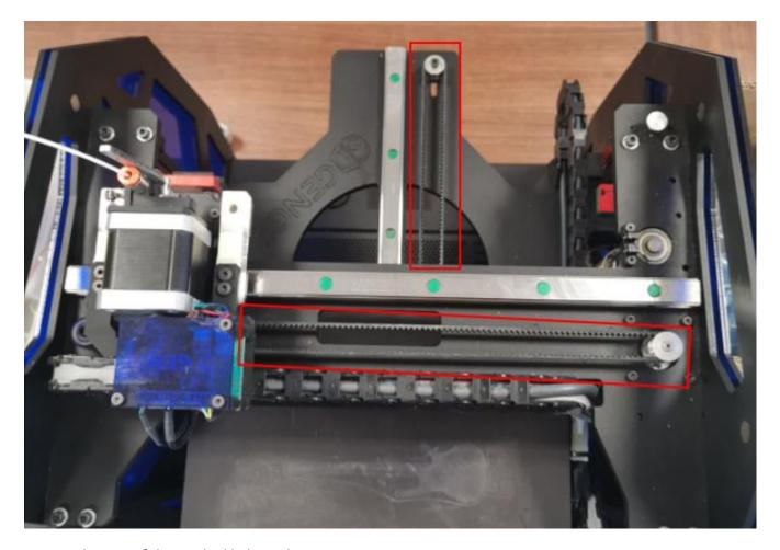
Fig. Localisation of the toothed belts in the printer.
