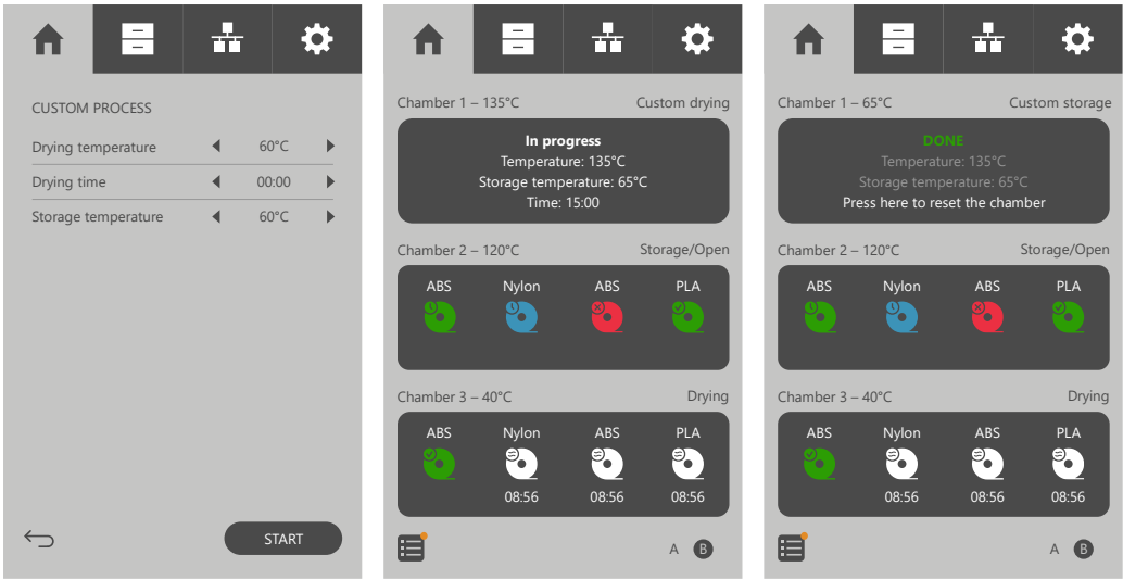
Fig. 48 Screens demonstrating the activation of the user-defined process
