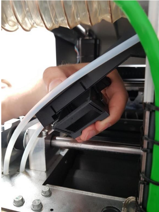
Fig. 116 The moment of cut-off of a fragment of the Bowden T0 tube
