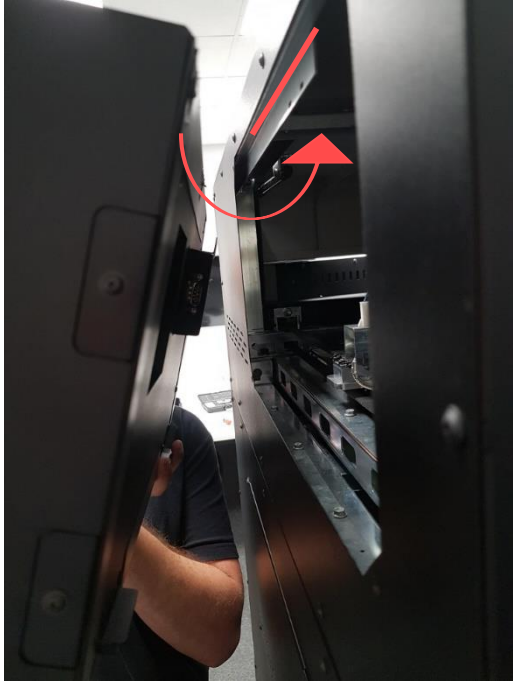
Fig. 123 Direction in which the FLEX accessory is slipped onto the printer
