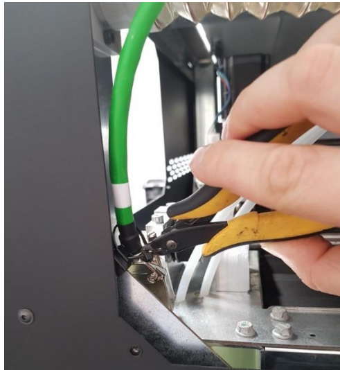
Fig. 113 Place to cut off the cable tie holding the connection cable to the accessory
