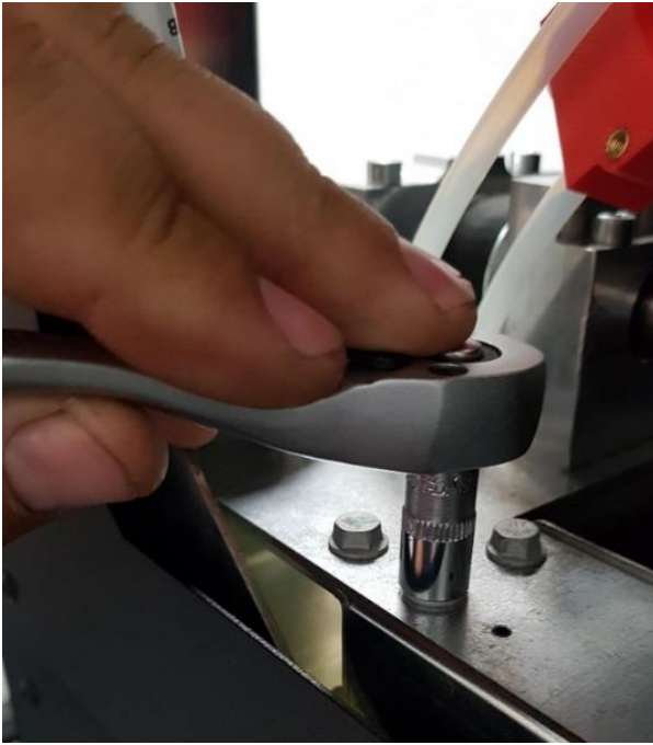
Fig. 120 Indication of the screw required to mount the Y-distributor bracket
