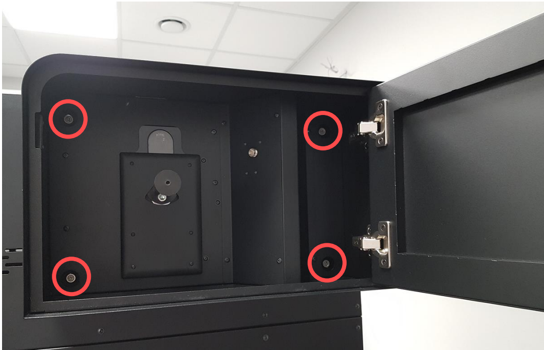
Fig. 125 Indication of the location of the mounting screws for the FLEX accessory
