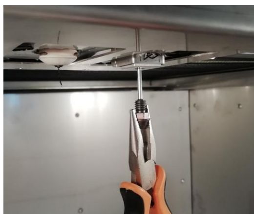
Fig. 91 Removing the hotend tip
