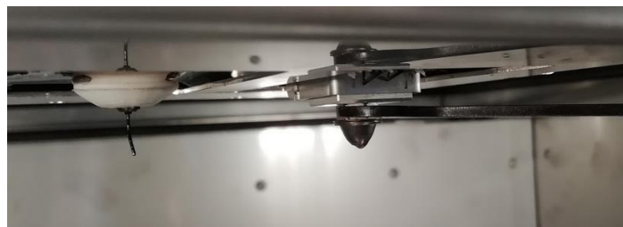
Fig. 90 Unscrewing the hotend tip
