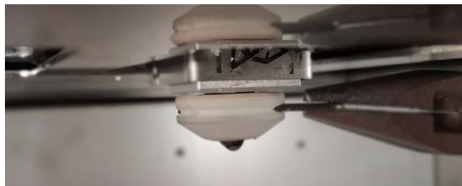
Fig. 93 Installing the metal cotter pin
