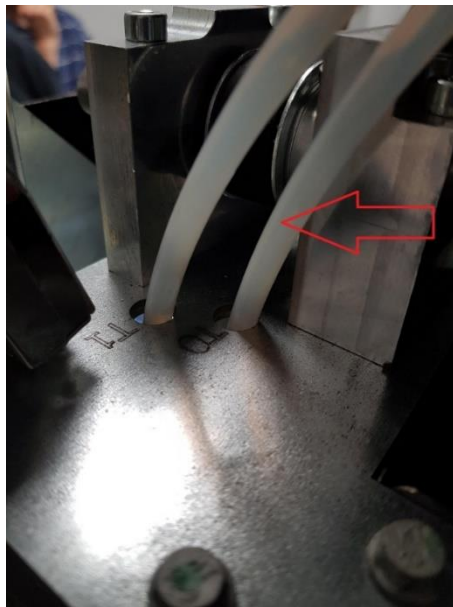
Fig. 114 Bowden T0 tube location
