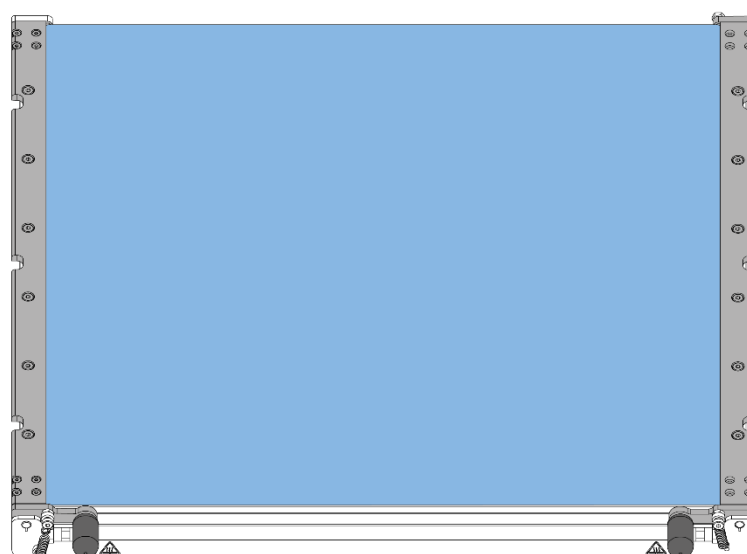
Fig. 75 Build plate installation – close clamps with handles
