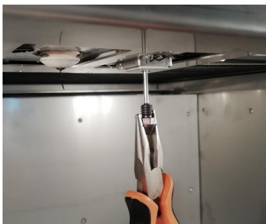
Fig. 92 Removing the hotend tip
