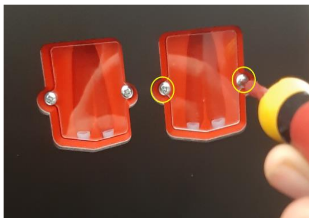
Fig. 127 Unscrewing the fixing screws of the glass pane of the access opening
