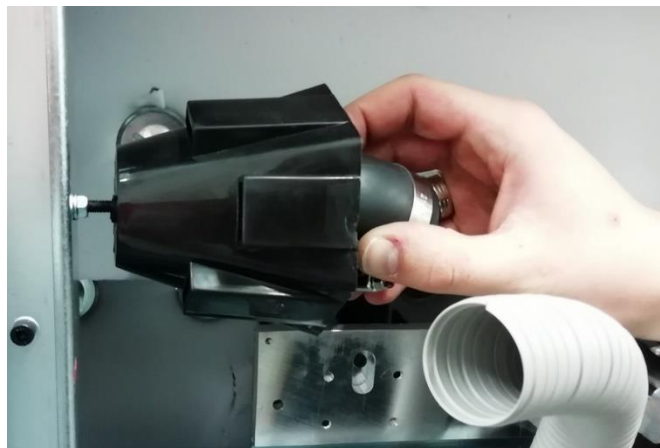
Fig. 123 Unscrewing and removing the filter element from the housing
