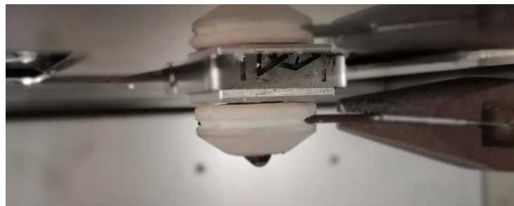
Fig. 94 Installing the metal cotter pin
